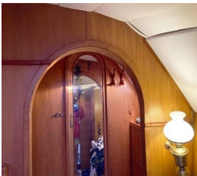
Reinforced cut out structural bulkhead port side
