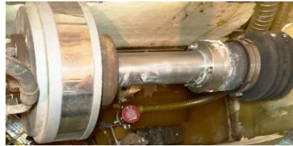
Volvo flexible coupling and rotating joint
