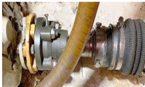
Perkins flexible coupling and rotating joint
