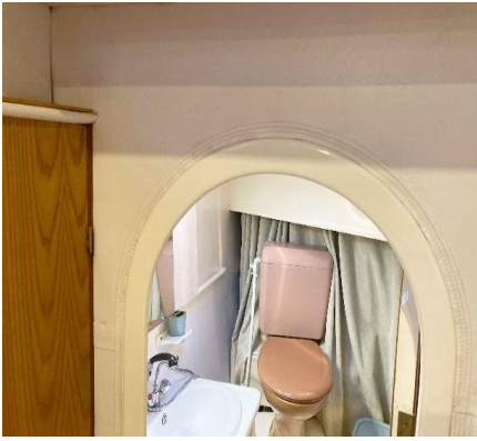
Reinforced cut out structural bulkhead aft side
