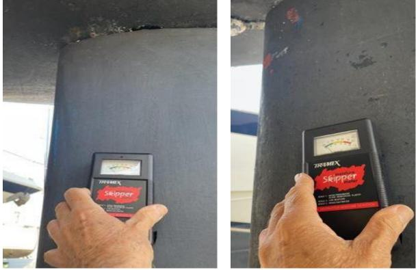
All sensitive areas of the 3 hulls – seacocks, shafts, rudders, keels - are free of osmosis/humidity except starboard rudder (slight moisture)
